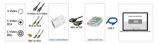
Detail of the connections based on the output video format:
