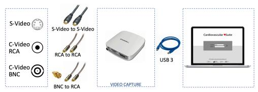
Detail of the connections based on the output video format:
