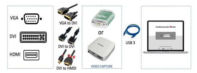
Detail of the connections based on the output video format:
